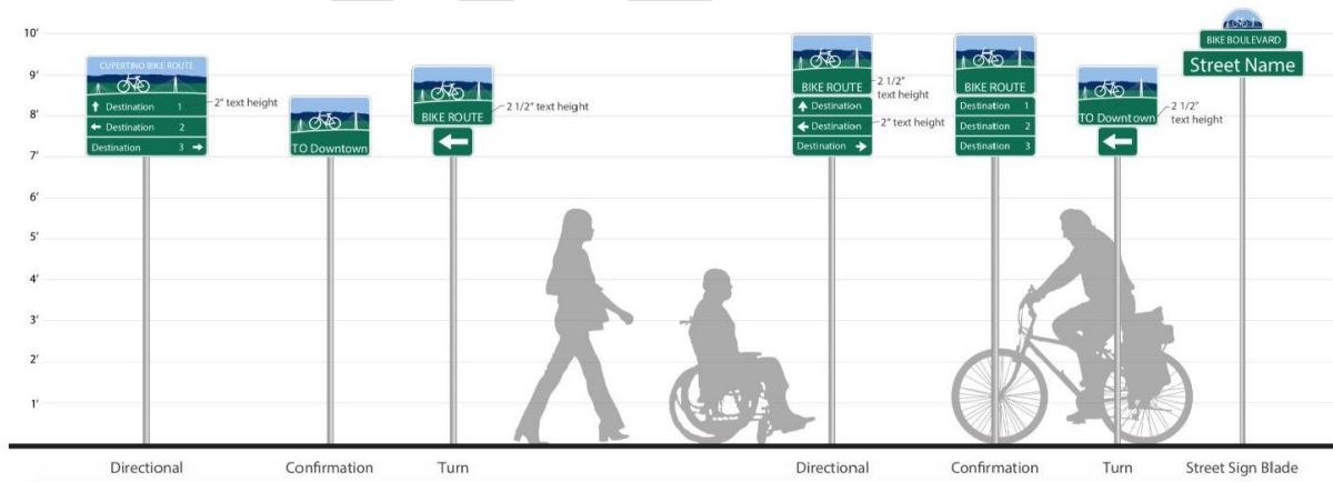
Figure 8-52 Representation of Wayfinding and Signage Boards Heights 46
